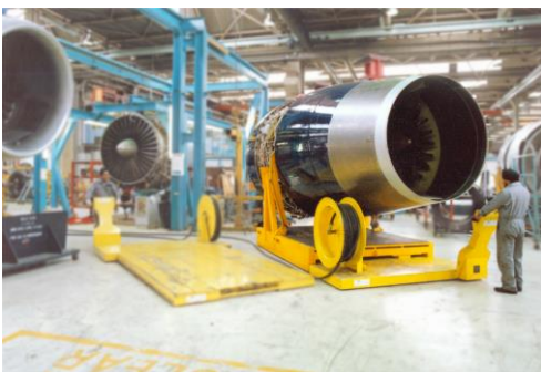
A single operator moves an Aero Engine on an air film transporter
