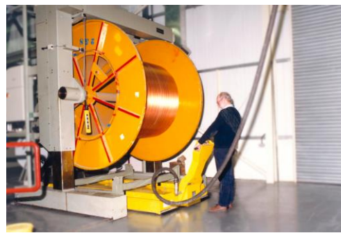
25,000kg fibre optic cable reels are accurately positioned on air
